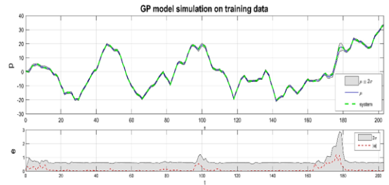
Fig. 4 GP model performance for the training signal. Upper part plots the true values, the predicted mean and 95 % confidence intervals, whereas below part shows the absolute residuals.
