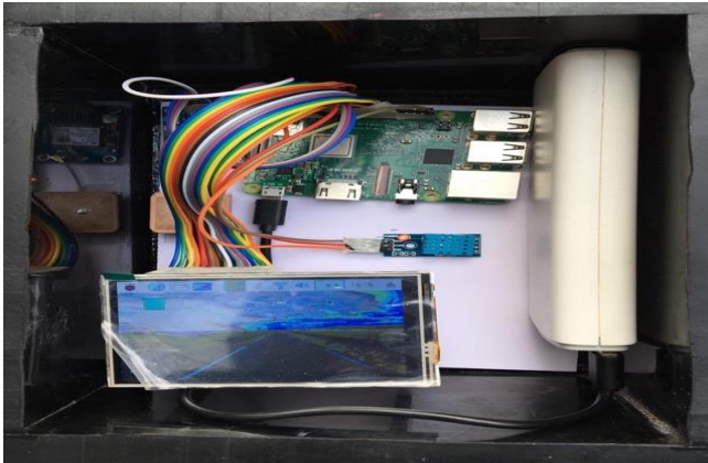
Fig 7. Hardware components of the non-localized sensor node
